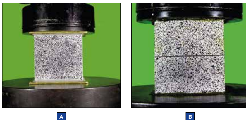
FIGURA 2 BOUNDARY CONDITIONS: (A) GLUED SHEETS, (B) GREASE
