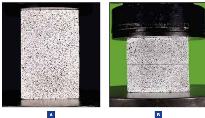
FIGURA 1 SPECIMEN GEOMETRIES: (A) PRISM, (B) CUBE
